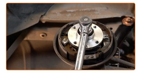
Tighten the hub. Use a drive socket #32. Use a torque wrench. Tighten it to 125 nm torque.
