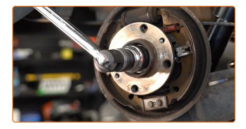
Unscrew the wheel hub axle nut. Use a drive socket #32. Use a tap wrench.
