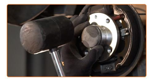
Install the hub bearing protection cap. Use a rubber mallet.
