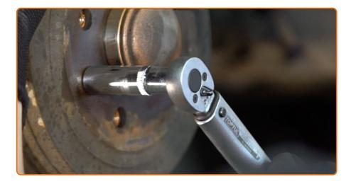
Tigten the brake drum fasteners. Use a drive socket #12. Use a torque wrench. Tighten it to 15 Nm torque.
