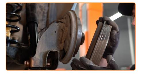
Remove the brake drum.
