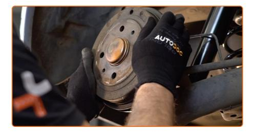
Install the brake drum and fasten it.
