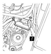
1. Move the section of front cable away from the work area.
