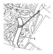
1. Check that the fluid level corresponds to the MAX notch on the reservoir.
