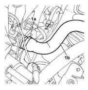
1. Disconnect the electrical connection from the braking system control unit.
