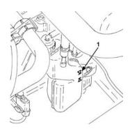
If the level is below the MAX mark, add fluid until the level is correct.
